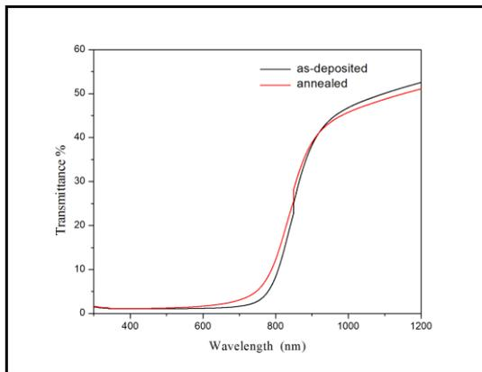
Figure 3: Transmittance spectrum of as-deposited and annealed film
