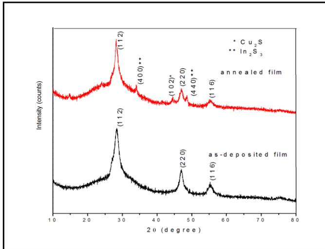
Figure 1. X-ray pattern of CuInS<sub>2</sub> thin film
