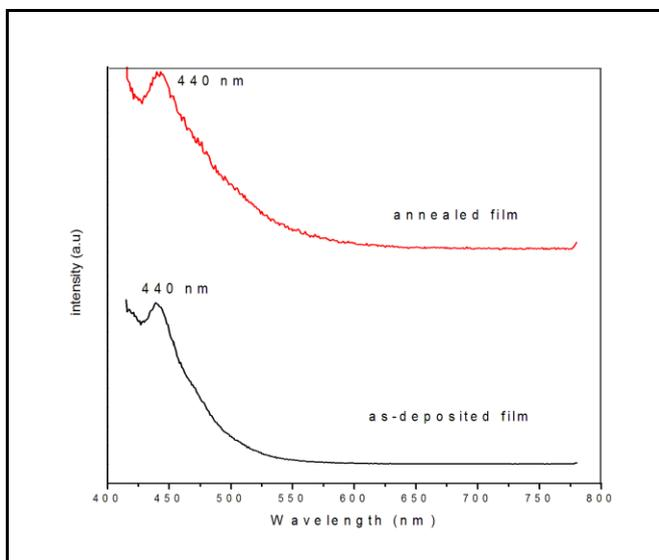
**Figure.6 Photoluminescence spectra of CIS thin film**
