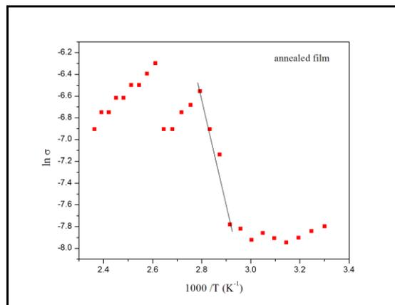
Figure 8. Arrhenius plot of annealed film
