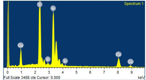
Figure 2. EDAX spectrum of CIS thin film
