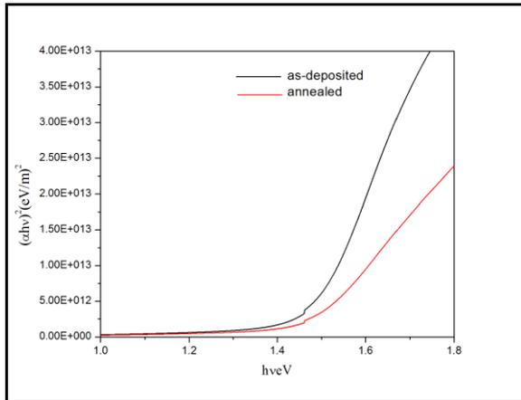
**Figure 5. Optical bandgap of as-deposited and annealed CIS film**
