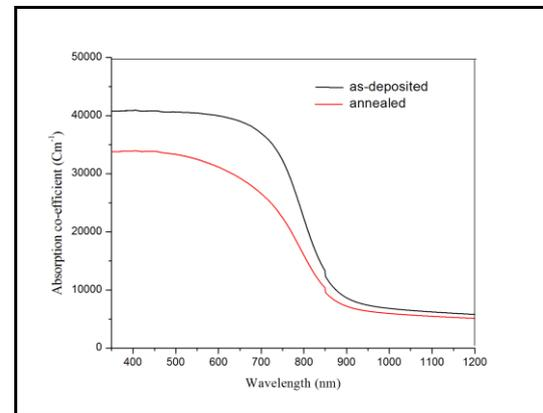
Figure 4: absorption co-efficient as a function of wavelength of CIS film
